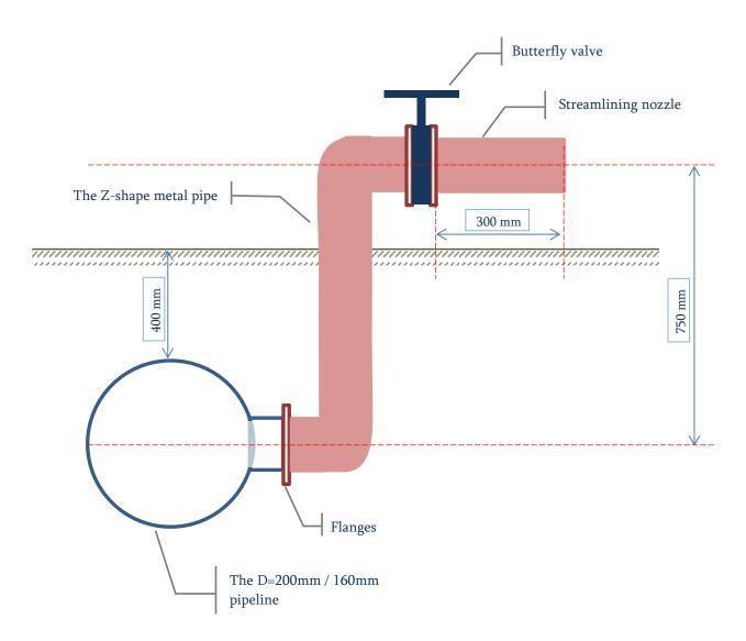
Schematics for connection of Z-shape pipes, 'butterfly' valves and 'streamlining nozzles'
