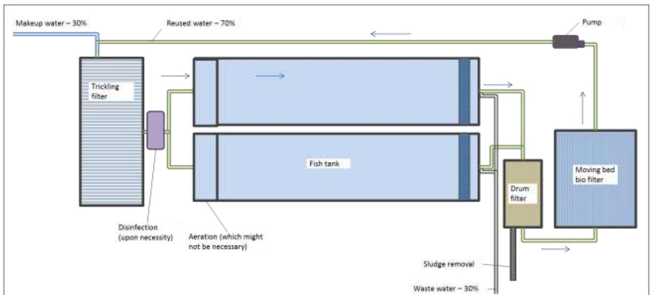
The model consists of two fish tanks, drum filter, moving bed bio filter (can be substituted by submerged bio filter), pump, trickling filter, disinfection block, and aeration.
