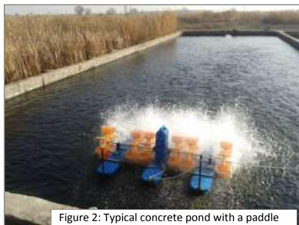
Figure 2: Typical concrete pond with a paddle wheel aerator (*Masis Region, v. Sipanik*)
