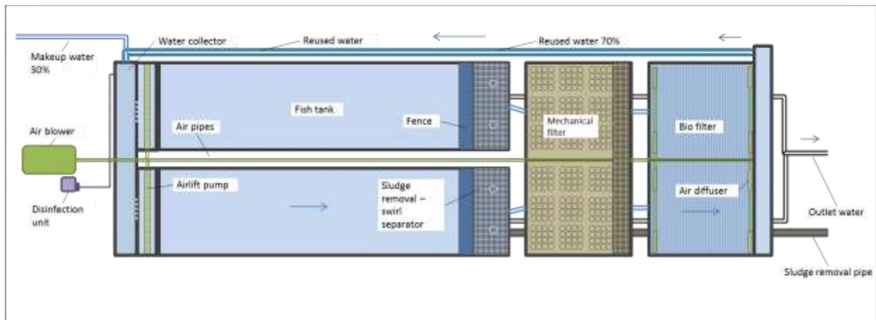
The model consists of two fish tanks, mechanical filter based on bio-blocks, moving bed bio filter, airlift pump, and disinfection block.
